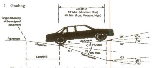
The shoulder slope usually varies from  $1/8^{\circ}/ft$ . (2%) to  $3/4^{\circ}/ft$ . (6%). However, the shoulder slope should be maintained when constructing theodrivewa<sup>D2</sup>.
